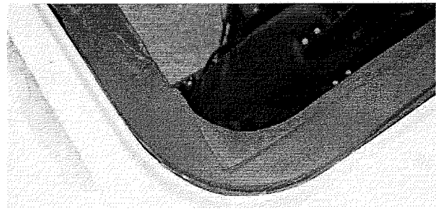
Weather seal with correct amount of lubricant:
